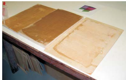
Bonding plywood to the prepared foam to make panels.
