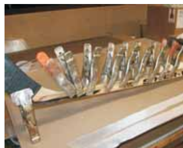
3. Clamp the stick together with even pressure to force a small amount of epoxy from the crack.
