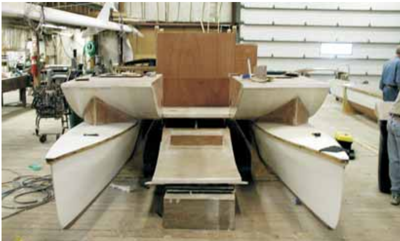
Gougmaran's bow showing the wave deflectors and the walk-on ramp in the down position.
