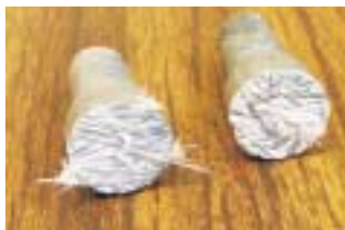
Pulled PATTI studs show that the failure was in the substrate, not in the gelcoat or the glue line.
