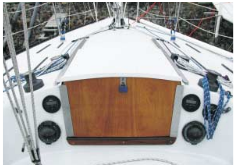
Left and below—The finished project. After two coats of Awlgrip™ Matterhorn white urethane, we masked off the areas we wanted to remain smooth. We mixed and applied a third coat thickened with 406 Filler to create the non-skid texture.
