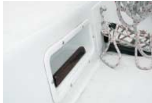
Left and below—The finished project. After two coats of Awlgrip™ Matterhorn white urethane, we masked off the areas we wanted to remain smooth. We mixed and applied a third coat thickened with 406 Filler to create the non-skid texture.
