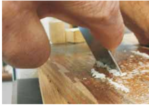
Left —The putty knife scraper used as a push scraper.
