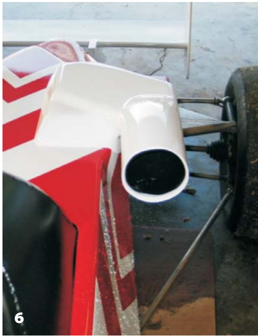
6—The finished air scoop viewed from the front. The lost foam method of composite fabrication was ideally suited for the scoop's aerodynamic shape.
