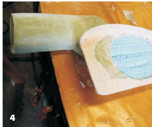
4—The cured part and mold from below before the foam was dissolved with lacquer thinner.
