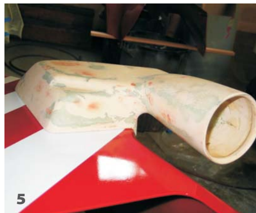
5—The cleaned up part after cleaning out the interior and fairing the exterior with epoxy/410 Microlight Filler.
